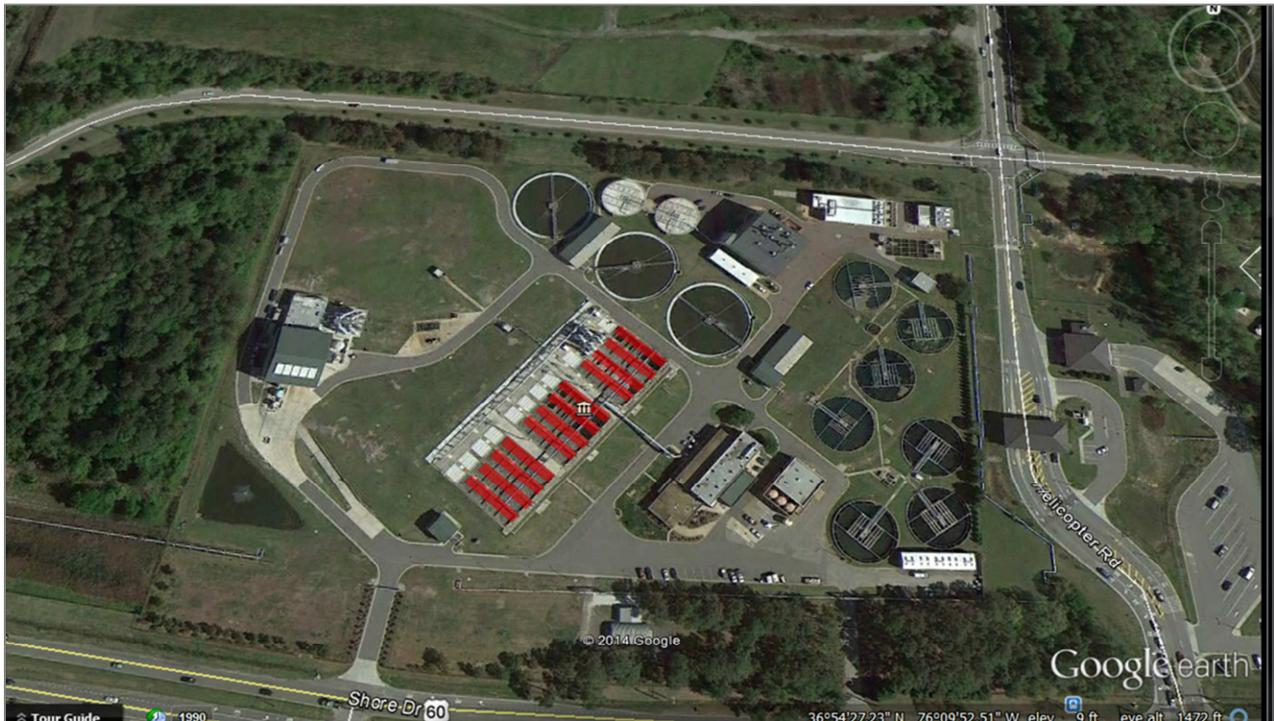
Figure 1 – Aerial View of the CETP with the Activated Sludge Biological Reactors in Red
