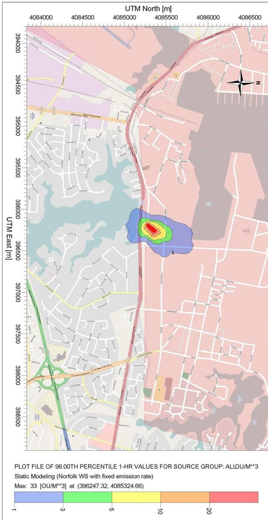
Figure 6 – 98th Percentile Concentrations for the Static Modelling Approach
