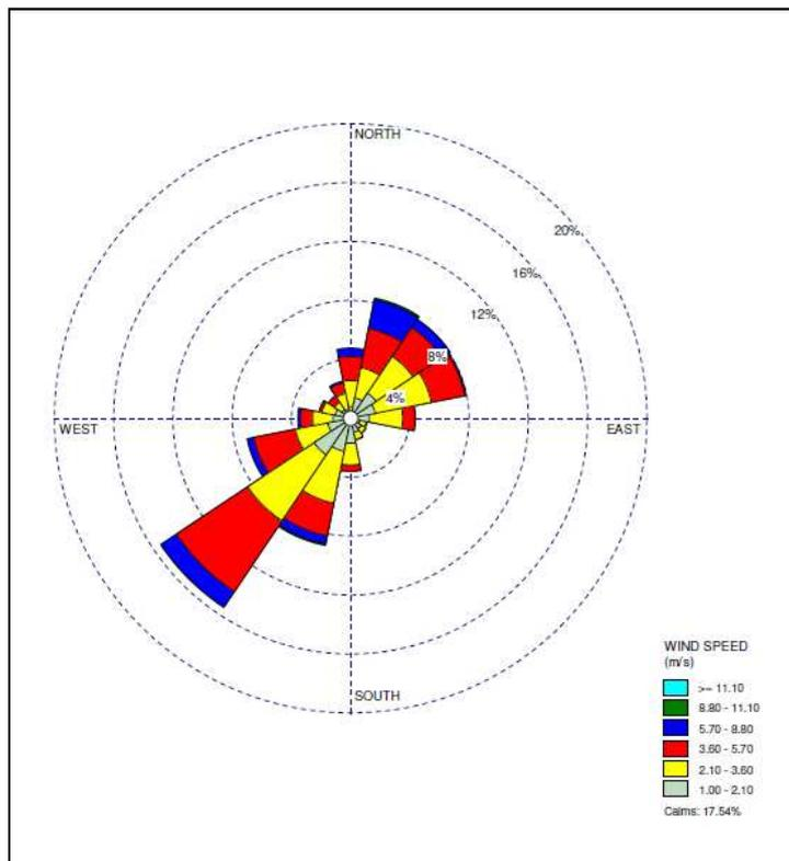
Figure 3 – Wind Rose of the On-site Station at CETP for 2013 (blowing from)
