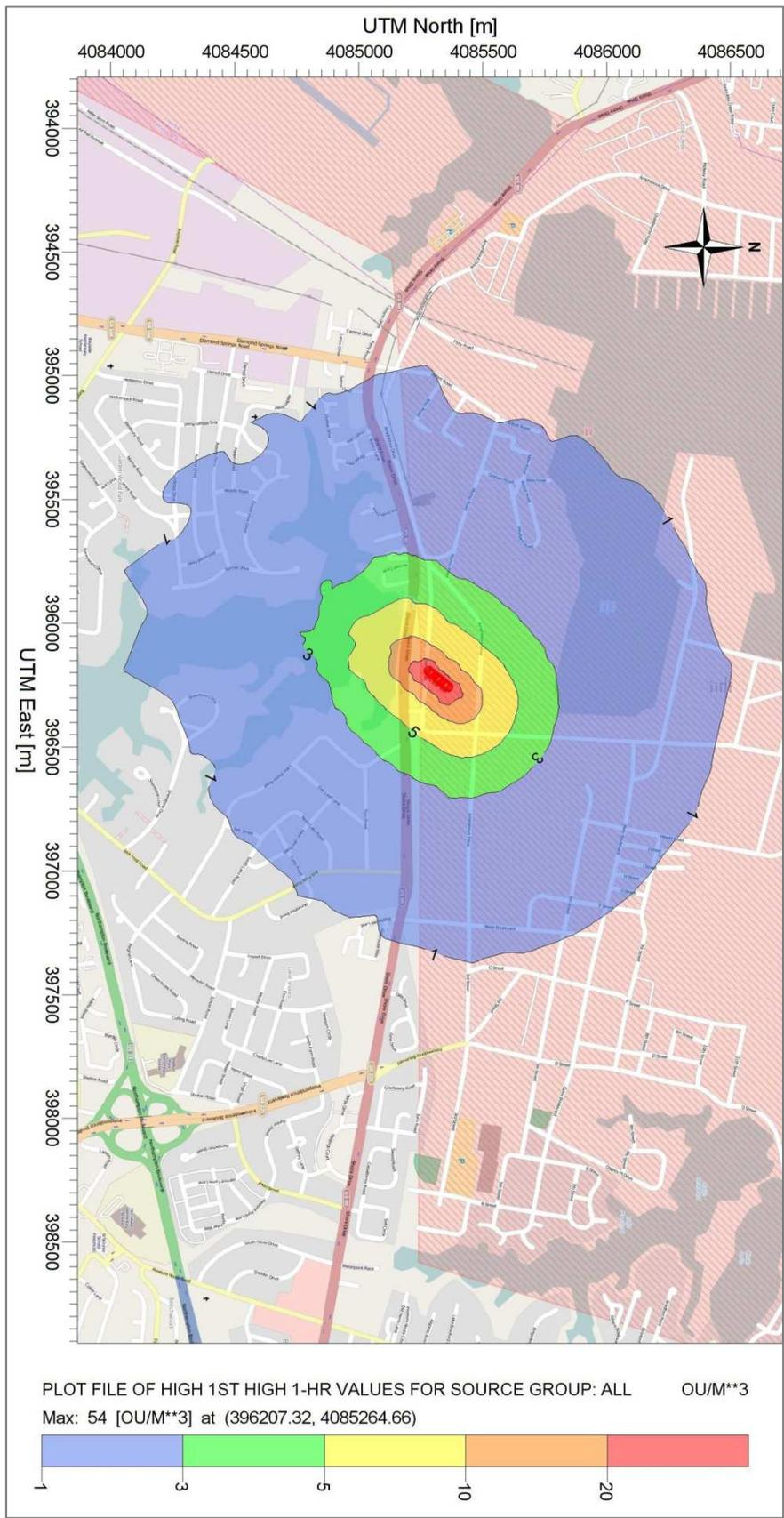
Figure 4 – Maximum Odour Concentrations for the Static Modelling Approach
